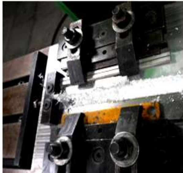
Fig. 2. Fixture holding plates for welding.
